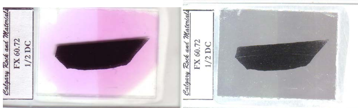
Figure 8. Thin Section of sample FX-60.72 under standard scan (left) and overexposed light (right) revealing subtle lamination within an organic-rich mudstone/shale.
