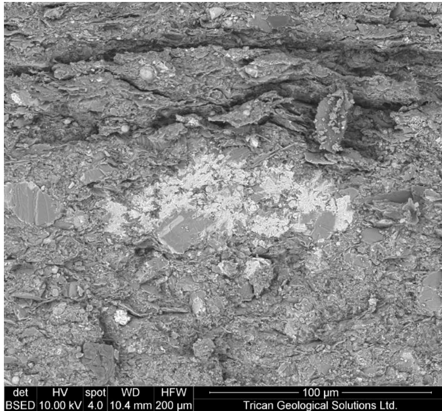
Figure 65. BSE photomicrograph showing lenses of barite cementation, intergrown with K-feldspar crystals.
